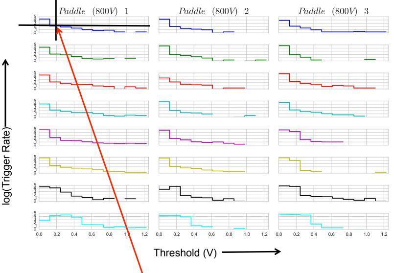
Set discriminator threshold via pre determined channel trigger rate
