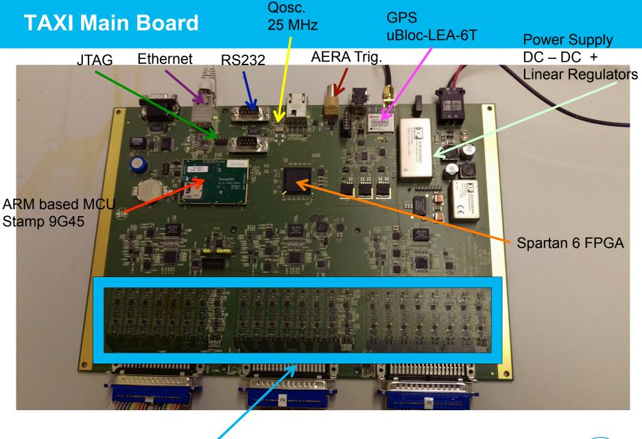
3 Scintillators X 8 discriminators per Scintillator = 24 channels
