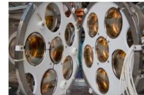
Setup to test 250 PMTs for XENON1T
