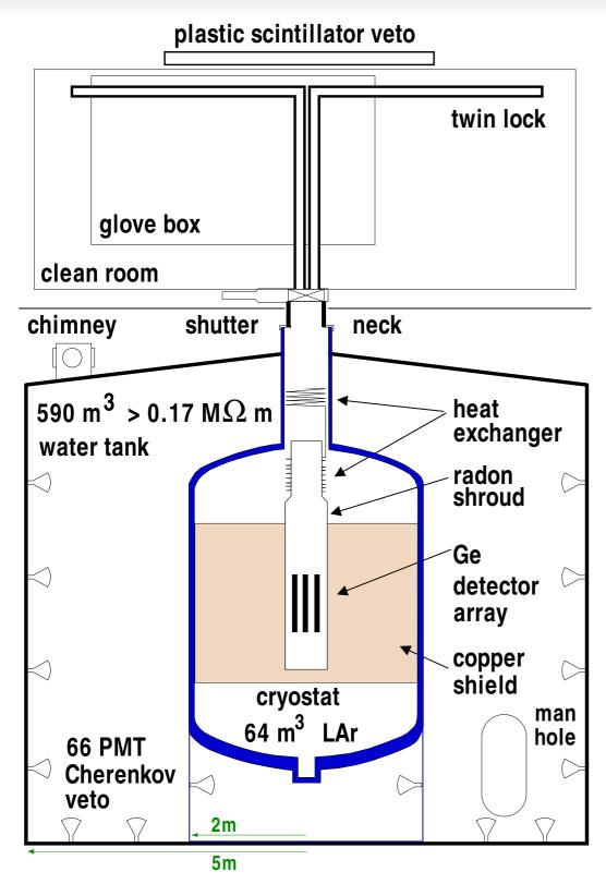
• 66, 8" PMTs in a ~600 m<sup>3</sup> water tank
