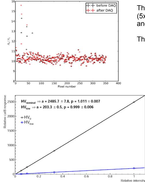
The ratio of calib. measurement A at the nominal  $(5x10^4)$  and reduced gain  $(5x10^3)$  before (black) and after (red) data taking.
