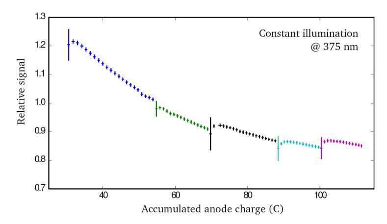
The PMT response as a function of the accumulated anode charge is shown above. After the initial aging phase the PMT response changes very slowly as has also been measured for PMTs operated at the nominal gain.
