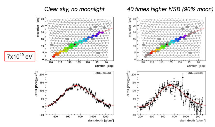
Figure 6.3: A real FD event with reconstructed energy  $7 \times 10^{19}$  eV. In the left panel are measured data (clear sky and no scattered moonlight, a baseline variance of 25 (ADC counts)<sup>2</sup>) and in the right panel the same data after adding random noise corresponding to a 40 times higher NSB.
