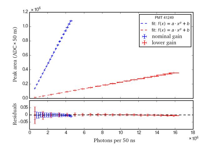
The PMT response to photon flux up to the saturation level measured at the nominal (blue) and reduced (red) gain. The exponent p is 1.0 for both gains.
