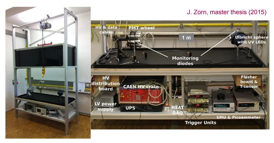
A uniform UV light source, which can be simultaneously operated in the DC and pulsed mode, illuminates FD PMTs. The FD electronics (20 MHz) is used to read-out measured signals.
