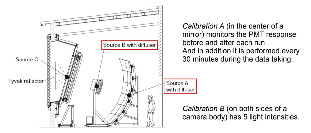
**Fig. 28.** A schematic showing positions of light sources for three different relative calibrations of the telescope.
