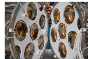
Setup to test 250 PMTs for XENON1T
