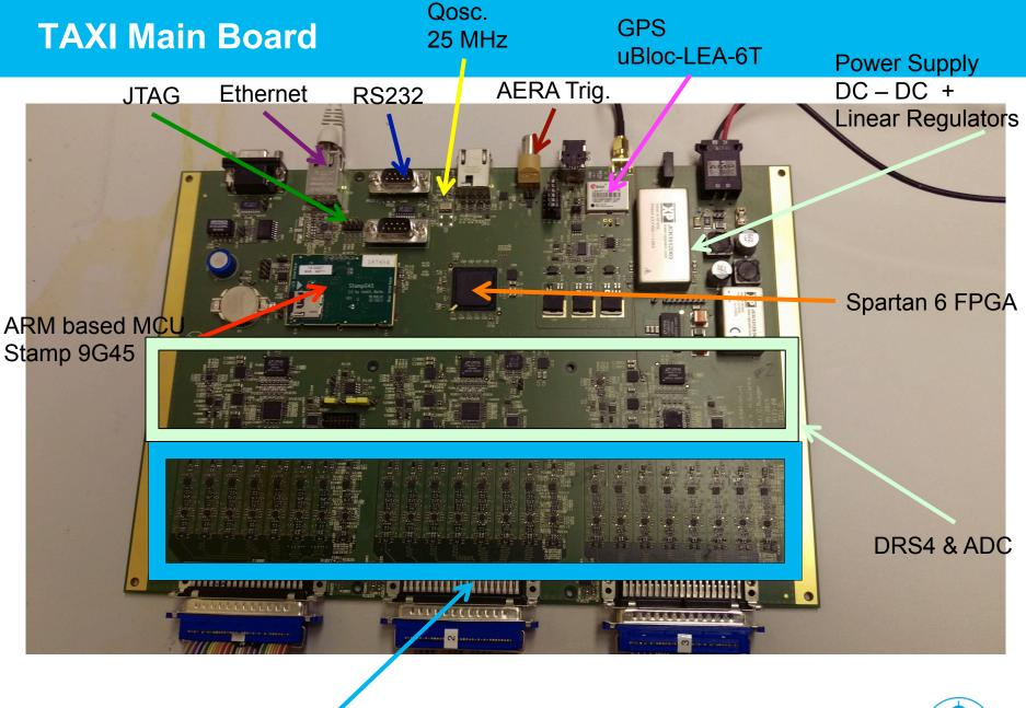
3 Scintillators X 8 discriminators per Scintillator = 24 channels
