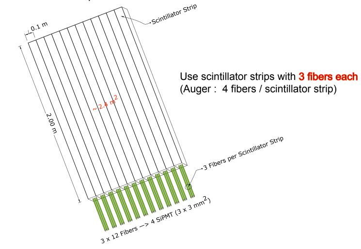
Cover ~ 2.4 m<sup>2</sup> with 12 scintillator strips And 4 3x3 mm<sup>2</sup> SiPMs
