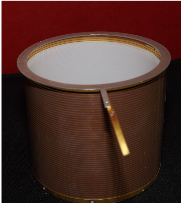
PCB for field shaping pitch: 1 mm
