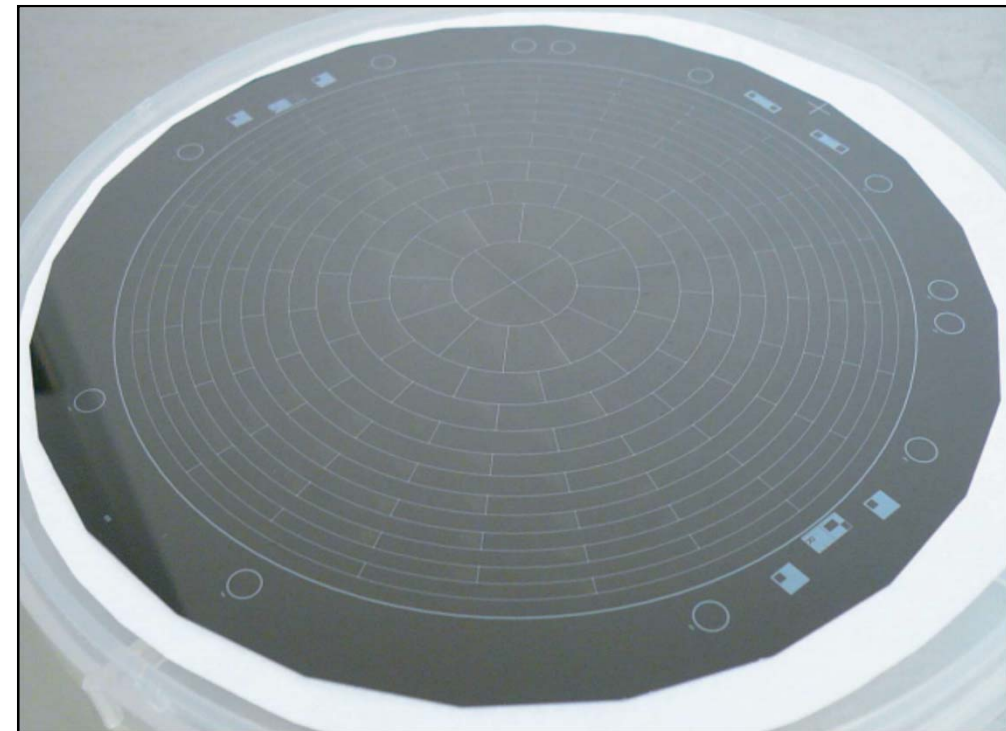
▲ detector wafer (segmented back side)
