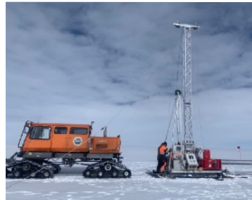
Drilling, installation of antennas at a depth of over 100 m
