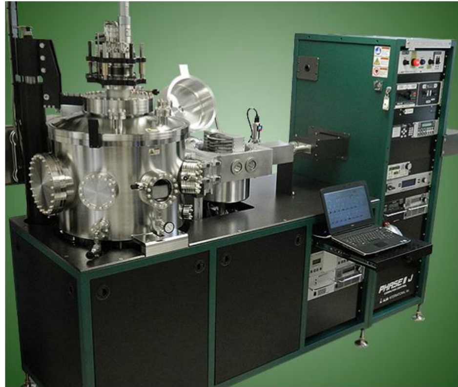
New 6 guns AJA ACT2400 sputter tool for superconducting films deposition. PO Sept. 2021. expected to arrive in Jun. 2022
