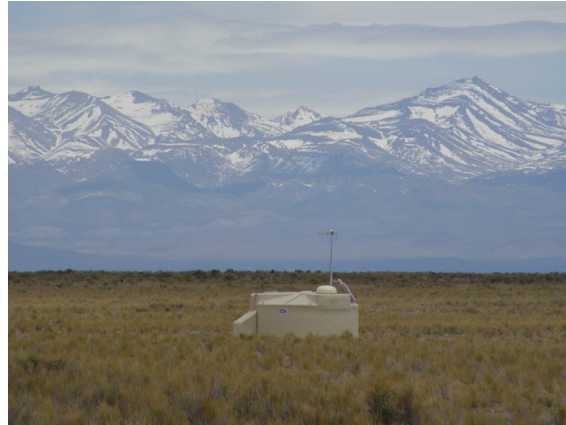
Surface Detector (SD) with 1660 stations
