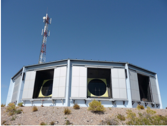
Fluorescence Detector (FD) with 27 telescopes
