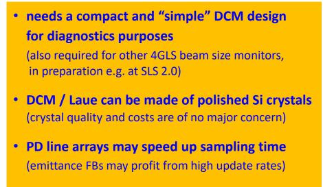
resolution can be improved for 4GLS beam profile monitor requirements by using Si (3,3,3) (...instead of Si (1,1,1) in SLS experiments)
