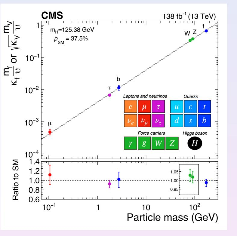
Higgs couplings to the most massive particles of the Standard Model measured remarkably well
