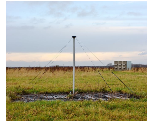
Low-band antenna, analyzed from 30-80MHz
