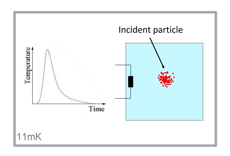
Crystal (TeO<sub>2</sub>) containing  $0v\beta\beta$ candidate (130Te) Kept at ~ 10mK **Energy deposition** increases temperature Detected with resistive thermometer μK sensitivity
