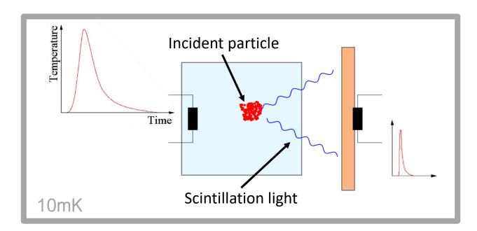
Cryogenic calorimeter used as light detector
