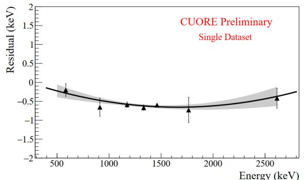
Energy bias due to imperfect calibration Fed to the fit as nuisance parameter
