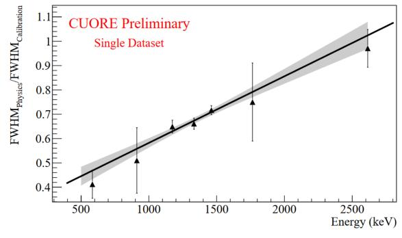
Energy resolution scales with energy Used to get the resolution at QValue
