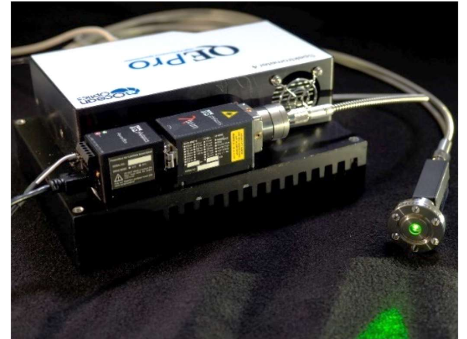
Figure – micro-Laser Raman system (F. Priester et al., Sensors 2022, 22, 3952; https://doi.org/10.3390/s22103952 )
