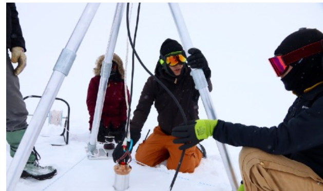
Melting probe in field 2023 to study refractive index
