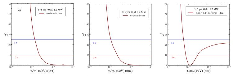
The figures show the sensitivity, discovery potential and measurement capability of DUNE for  $\tau_3/m_3$  from left to right. DUNE can put bound on neutrino lifetime of  $\tau_3/m_3 > 2.38 \times 10^{-11} (s/eV)$ . DUNE can discover neutrino decay at more than  $3\sigma$  for  $\tau_3/m_3 < 2 \times 10^{-11} (s/eV)$  and for true  $\tau_3/m_3 = 1.2 \times 10^{-11} (s/eV)$ , the expected precision will be  $2.63 \times 10^{-11} > \tau_3/m_3 > 7.62 \times 10^{-12} (s/eV)$
