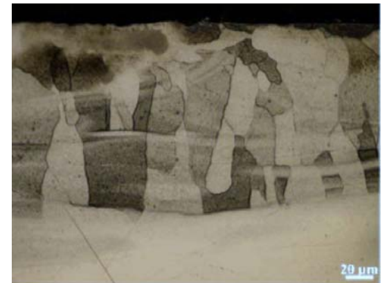
Weld overlay thickness: 210-220 μm Excellent ductility: bend test 180°
