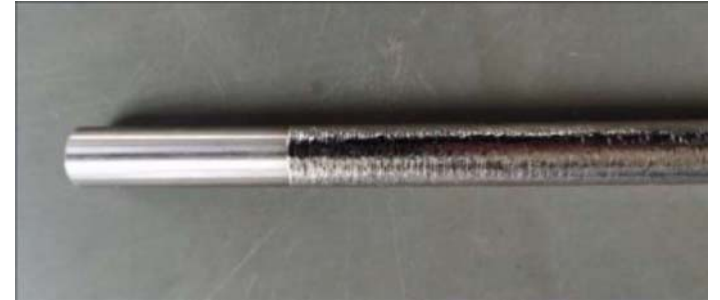
AISI 316L tube with weld overlay (Fe-10Cr-4Al-RE)
