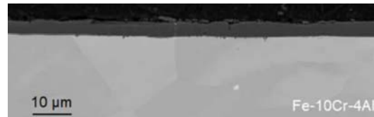
Fe-10Cr-4Al-RE: Exposed to liquid lead at 800°C, protective self-healing alumina
