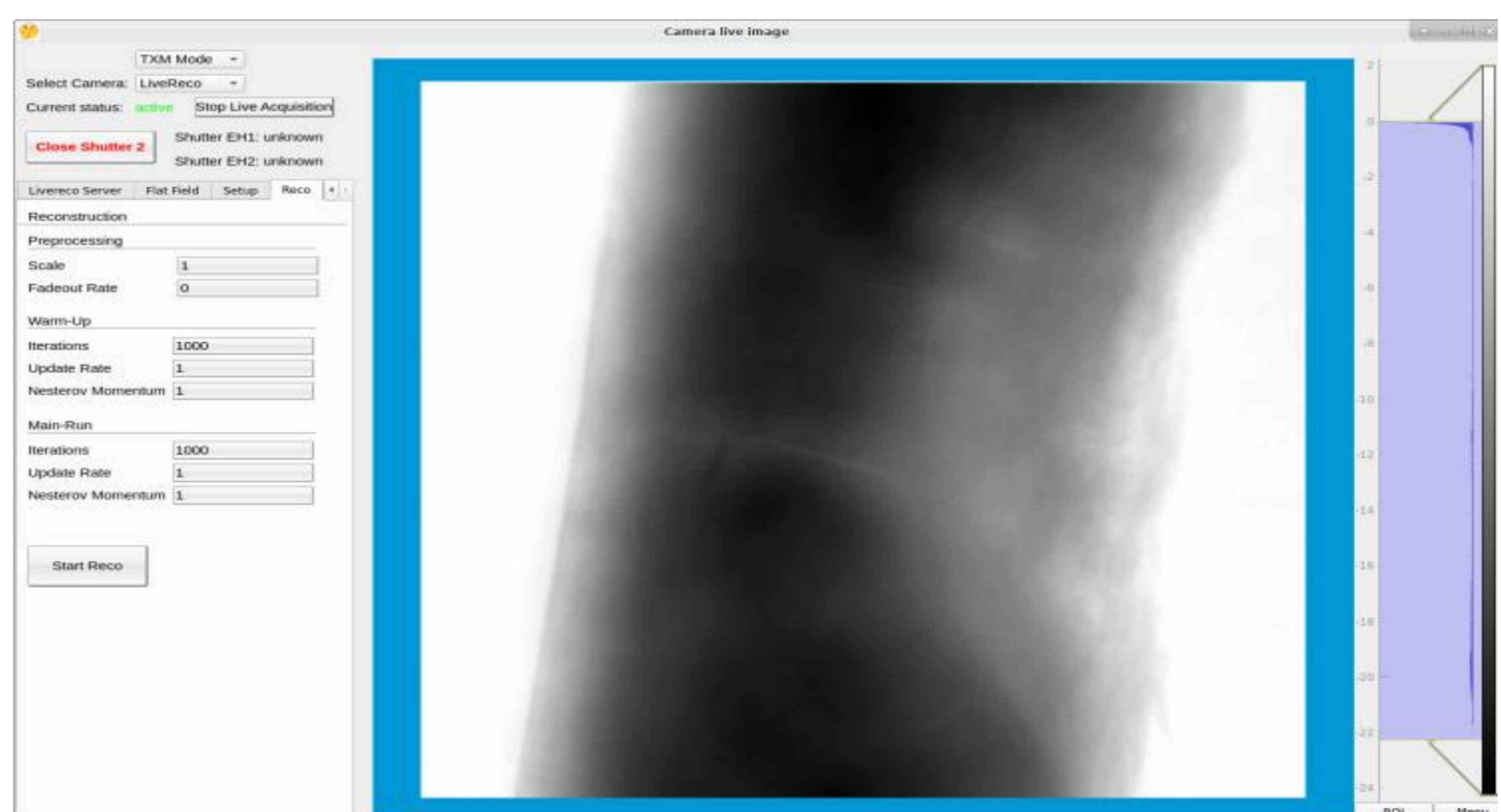
Fig. 3: Current user interface from P05 beamline. Showing the phase retrieved hologram. The phase retrieval algorithm takes approximately 40 seconds to obtain this result.
