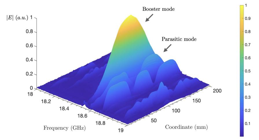
Identification of correct mode vie "bead pull measurements"
