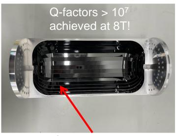
Coating with high *Tc* superconductor
