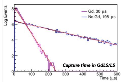
H produces a 2.2 MeV  $\gamma$ , Gd produces 4-5  $\gamma$ s totaling ~8 MeV
