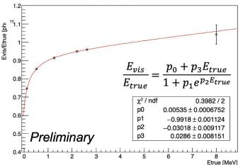
$E_{true}$  is the true energy deposited in the GdLS  $E_{vis}$  is the visible energy accounting for nonlinear GdLS response
