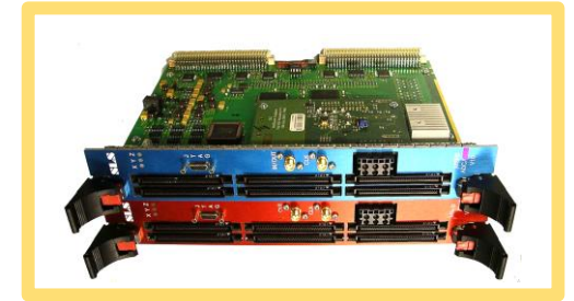
VME-based ADC/DAC cards with FPGA
