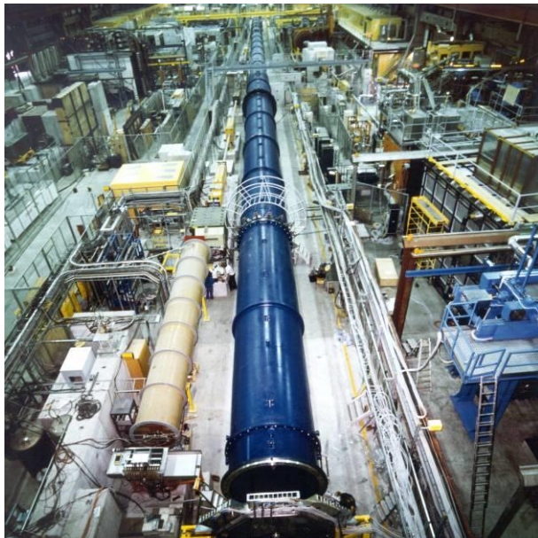
The 160m long NA31 decay tube and helium tank
