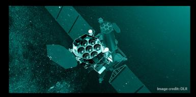
eROSITA – X-ray telescope
