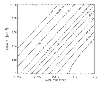
Figure 1. Stochastic-acceleration time-scale  $\tau_{\text{FII}}$  (equation 4) for an electron with  $\gamma = 10^4$  as a function of plasma number density *n* and the magnetic-field intensity *B* in ionized hydrogen plasma. Time-scales vary from years
