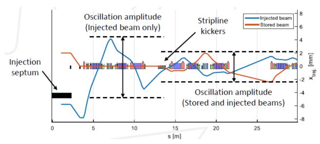
'Trajectory of injected- and stored bunch centroids through the first achromat during single-bunch aperture sharing. Chicanes are set to a 2 mm static bump.'
