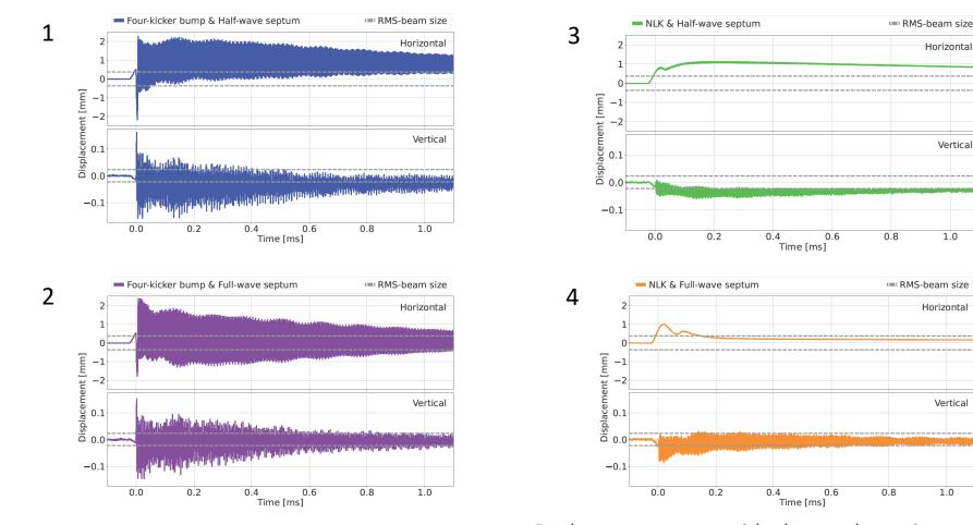
*Real measurements with electron beam in a storage ring:* Combination of full wave septum and non-linear kicker injection shows Kicker at BESSY II', Proc. IPAC'23, Venice, Italy, May 2023, pp. 1156–1158. the least beam displacement or excitation during the injection process.
