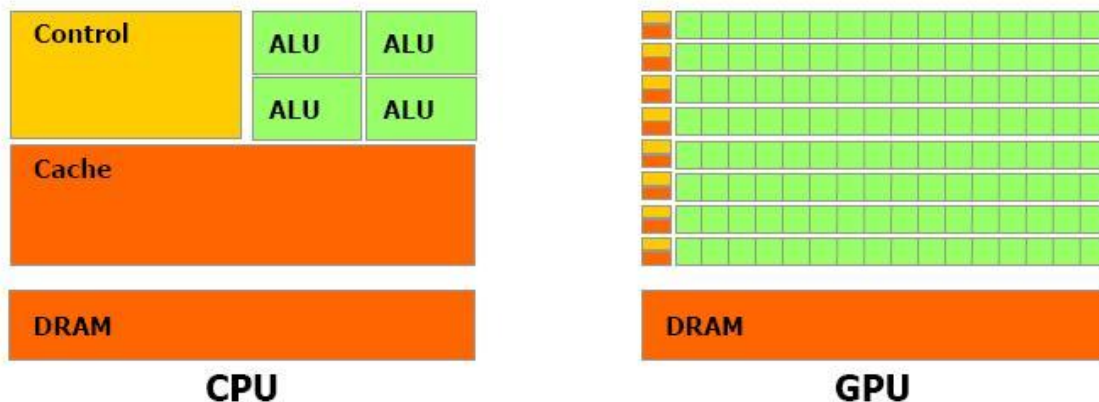
Figure 1. An NVIDIA illustration [25] of the potential computational power of the CPU by showing the relative ALU densities between CPUs and GPUs
