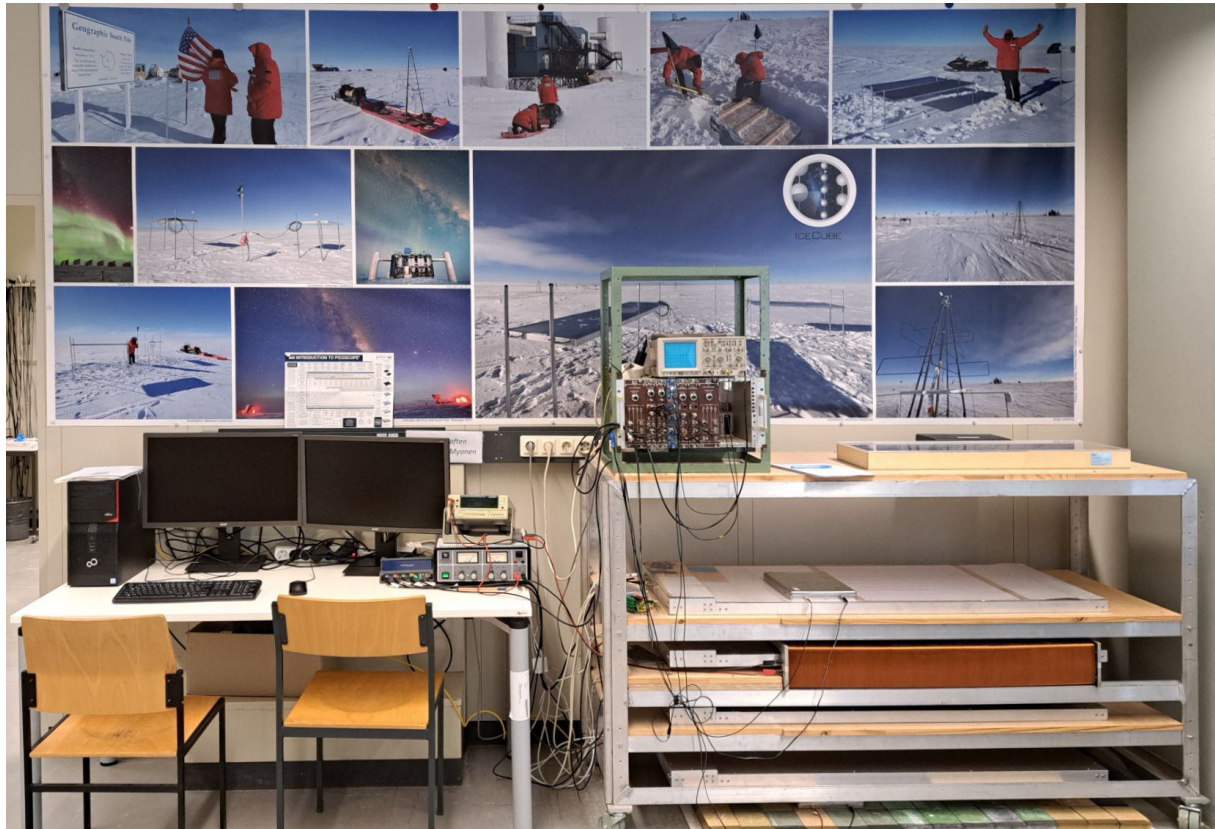
Figure 7.43: Setup of the cosmic muon experiment. The stack of three scintillation panels is seen on the right side. On the left side, the data acquisition electronics and the analysis computer can be seen.
