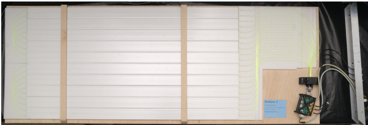
Figure 7.46: Scintillator module with ten scintillating bars, Si-PM, and electronics.
