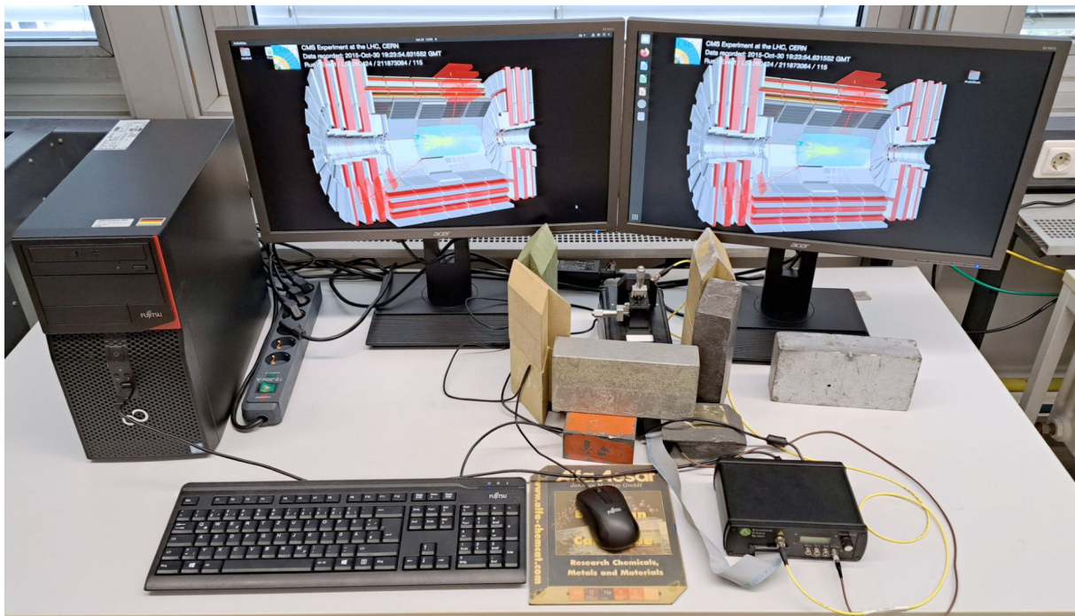
Figure 7.18: The Si-strip detector, investigated in this experiment is located in the black housing behind the lead shielding.
