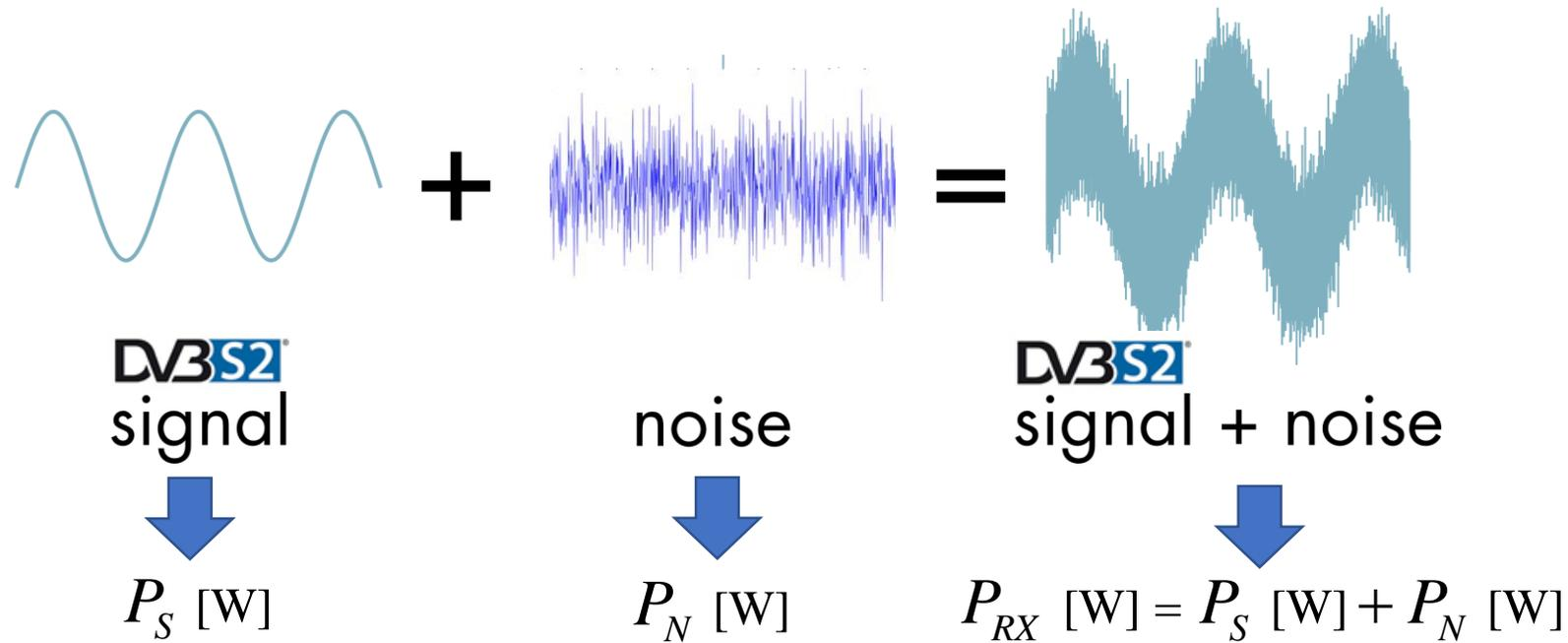
Commonly-used RF signal metric for the **Received Signal Level (RSL)**
