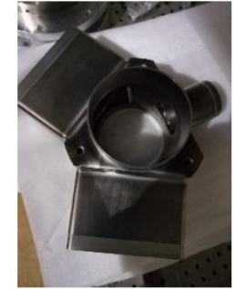
650 MHz 5-cell cavity with waveguide HOM coupler
