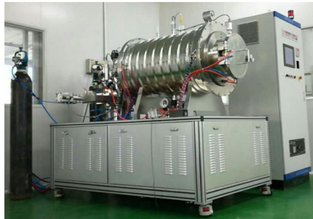
New furnaces for N-doping and infusion study
