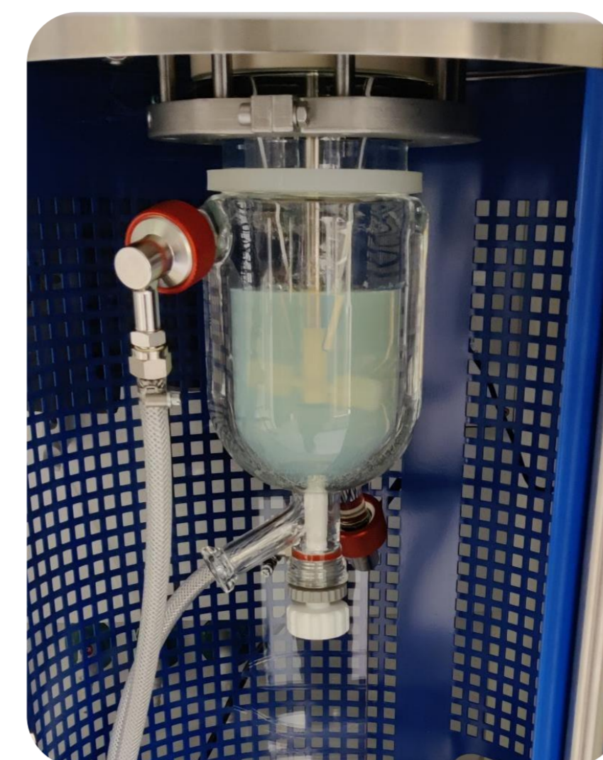
Figure 1: Reactors for the scale-up of lab polymer synthesis with volumes of 0.5 L, 2 L and 15 L.
