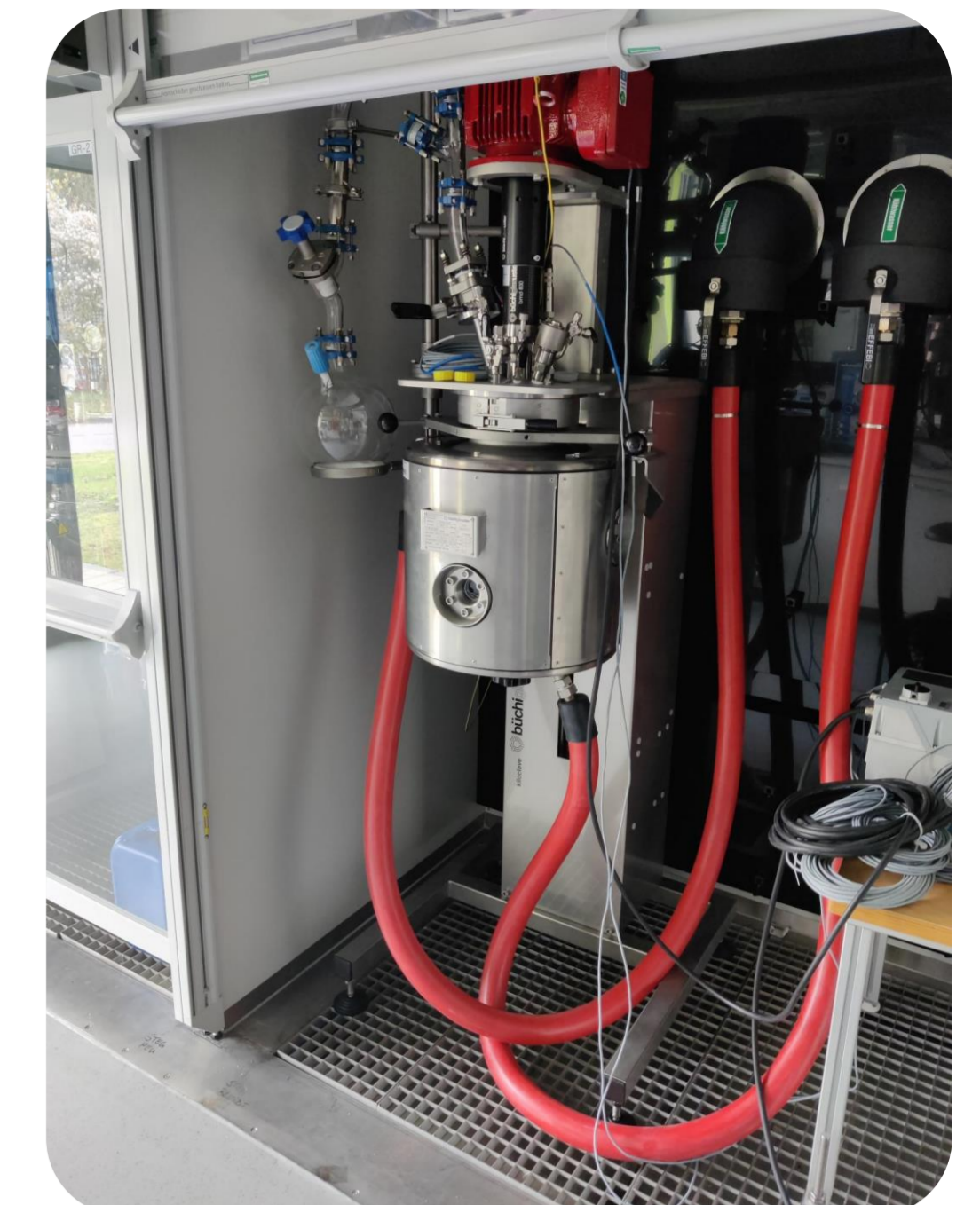
Figure 1: Reactors for the scale-up of lab polymer synthesis with volumes of 0.5 L, 2 L and 15 L.
