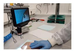
3. Adjust kapton into place under microscope
