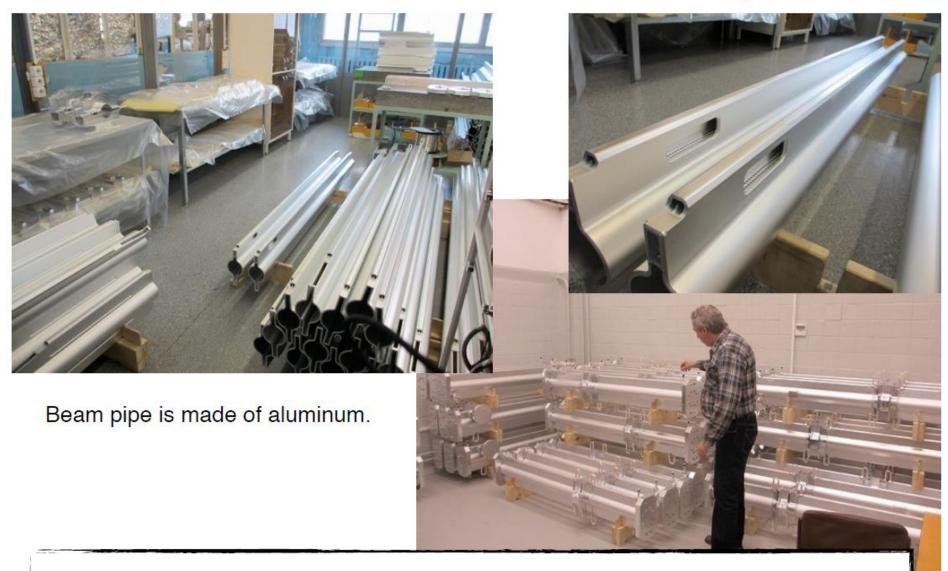
Fabrication of the LER arc beam pipe section is completed
