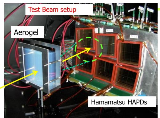
RICH with a novel "focusing" radiator – a two layer radiator
