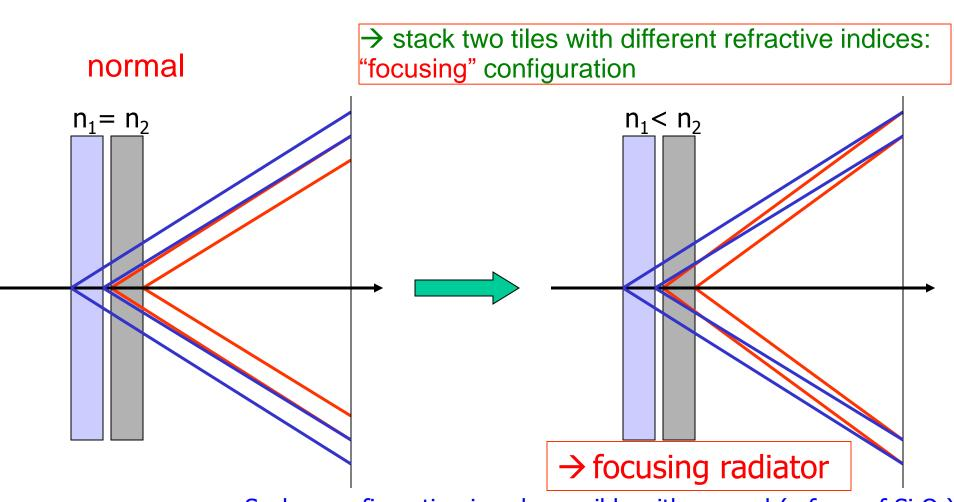
Such a configuration is only possible with aerogel (a form of Si<sub>x</sub>O<sub>y</sub>) – material with a tunable refractive index between 1.01 and 1.13.
