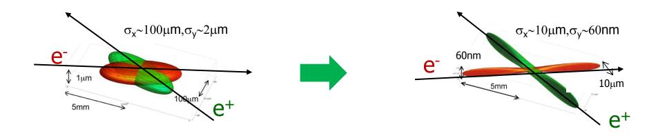
... For a 40x increase in intensity you have to make the beam as thin as a few x100 atomic layers!
