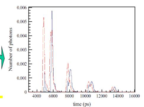
Time distribution of signals recorded by one of the PMT channels: different for  $\pi$  and K (~shifted in time)
