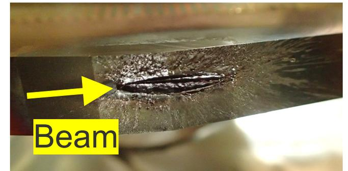
Vertical collimator was scraped off (LER)
