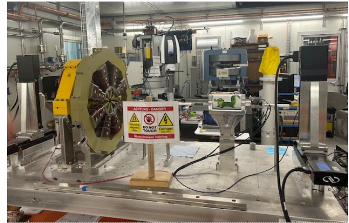
Sextupoles & Octupoles axis measurement with vibrating wires Team of 4 persons
