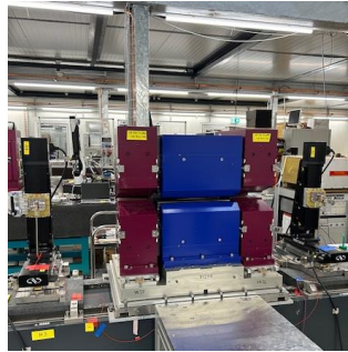
Triplet alignment vs. the nominal axes (survey group) + final tuning
