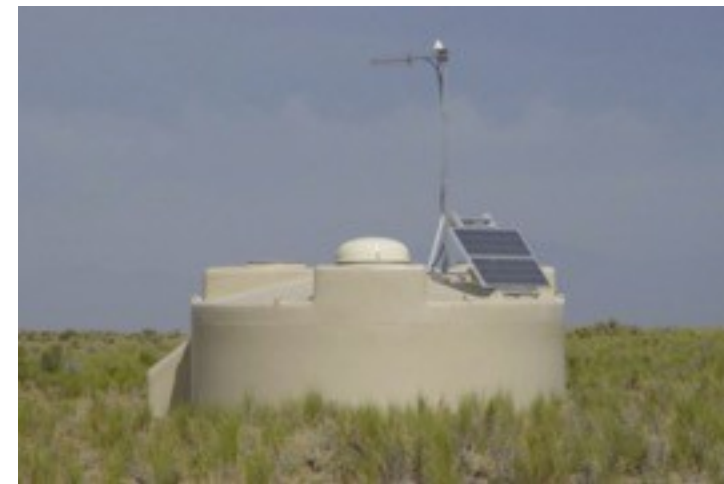
Surface Detector (SD) 1660 water-cherenkov detectors 100% duty cycle
