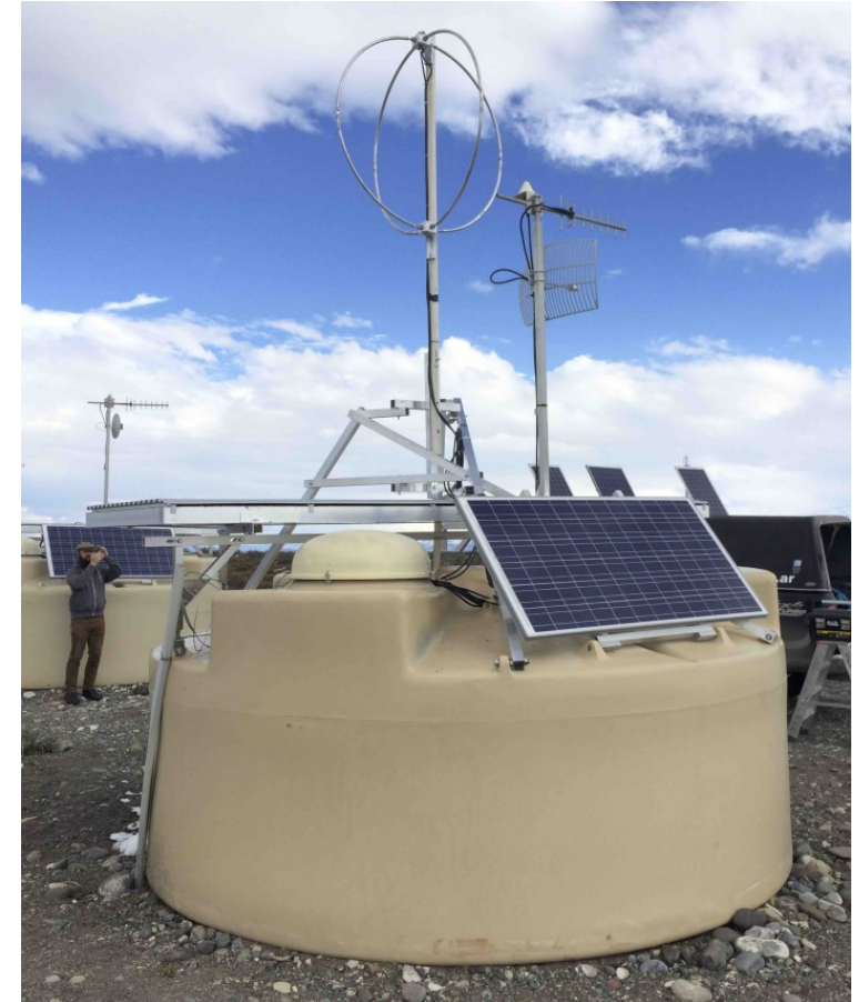
Prototype antenna installed in the AugerPrime engineering array
