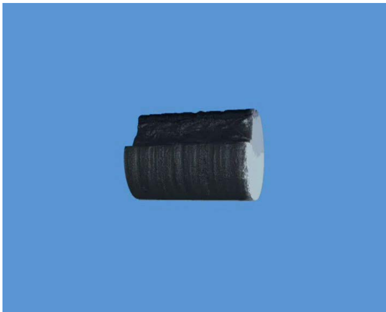
X-ray tomographic reconstruction of laser beam weld
