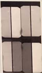
Fig. 1: Multi-filter raw image mosaic for g , r , i , z . The arrangement contains 8 CCDs, two for each filter.
